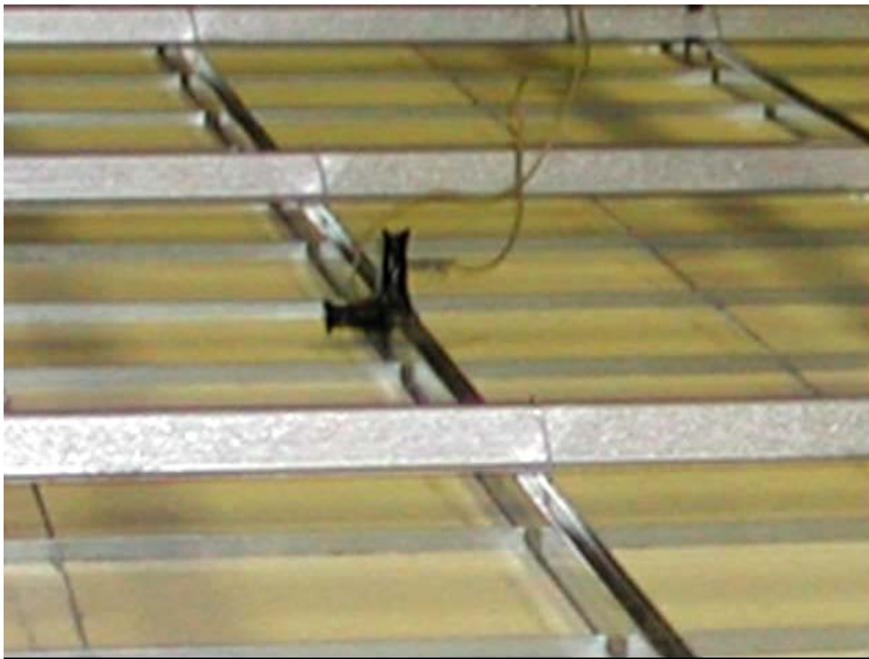
Figure 2–12b. Accelerometers monitoring the response of the test assembly on the ceiling support grid.
